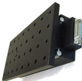
The LS-100's top plate has seventeen tapped and eleven countersunk 1/4" holes on 1" centers.
