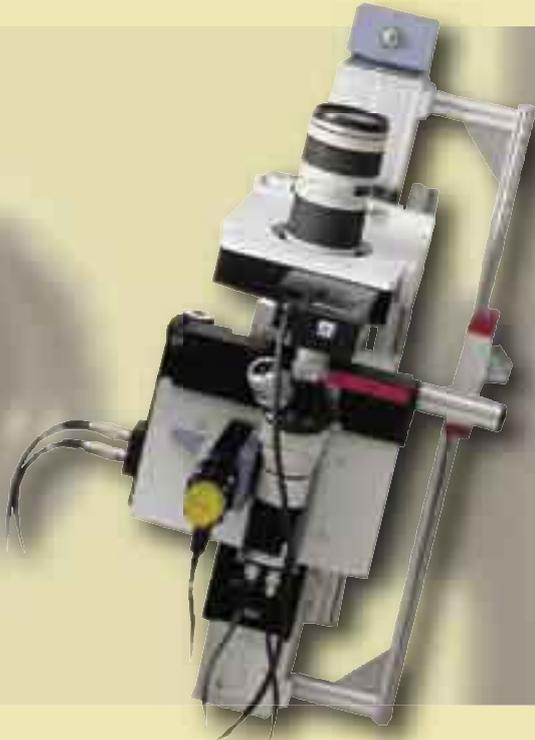
The modulation transfer function (MTF) is a recognized control criterion for the optical imaging quality. It characterizes the resolution of optical systems on the axis and in the image field. Beside the MTF with MTF Variant can be measured e.g. also the focal length, chromatic aberrations or the distortion.
