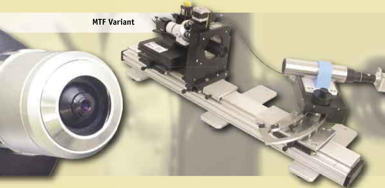
in imaging quality because of manufacturing errors. Because of the growing demands in imaging performance of lenses their characterisation by help of the Modulation Transfer Function (MTF) as the premier parameter for objectively evaluating is more and more used.
