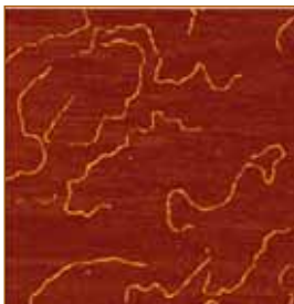
Typical AFM image of the DNA test sample (obtained in contact mode, humidity 1-10%, Solver BIO, NT-MDT Co.).
